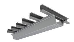
RFI 22 mm Ceiling Batten is manufactured using TRUECORE® steel (aluminium/zinc alloy coated) complying with AS1397 G550, AM150 (550 MPa minimum yield stress). Also available in Zincalume® steel
